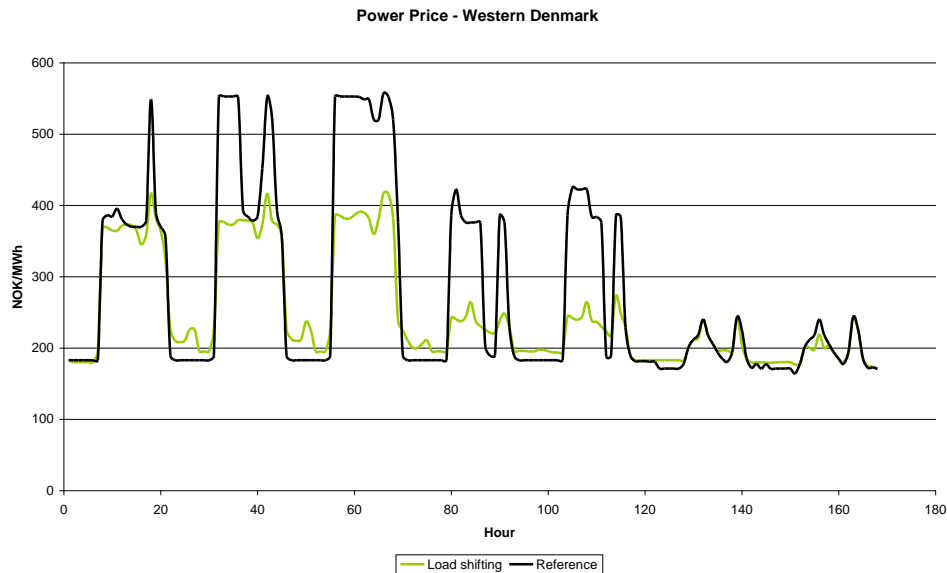
Figure 12: Example, load shifting scenario, high demand and low wind: Electricity prices in Western Denmark simulated for week 5.
