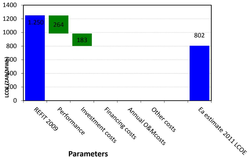
Figure 3: Influence of performance and investment costs on LCOE for wind power in 2011 compared with REFIT 2009.
