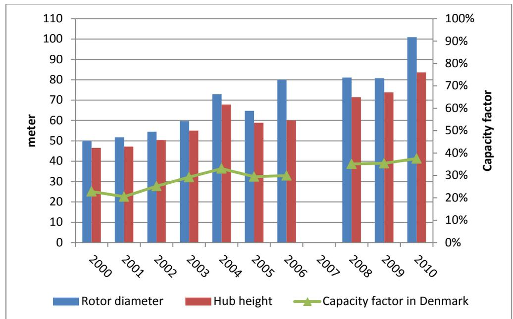
Figure 1: Development in average rotor diameter, hub height and capacity factor for onshore wind turbines commissioned in Denmark between 2000 and 2010 based on generation data for 2010. (No turbines commissioned in 2007)
