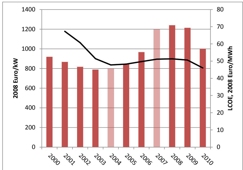
Figure 2: Average costs per kW for wind turbines commissioned in Denmark (columns) compared to development in average LCOE for wind power projects commissioned in that year (line) in Denmark. Data for 2004 and 2007 are estimates based on offers made to developers as no project cost data could be accessed for commissioned projects.
