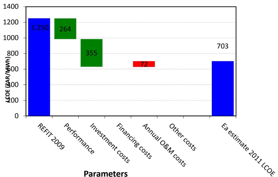
Figure 4: Influence of different parameters on LCOE for wind power in 2011 compared with REFIT 2009. The green columns indicate parameters that have reduced the 2011 LCOE compared with REFIT 2009, whilst the red columns indicate parameters that increase LCOE 2011 compared to REFIT 2009.
