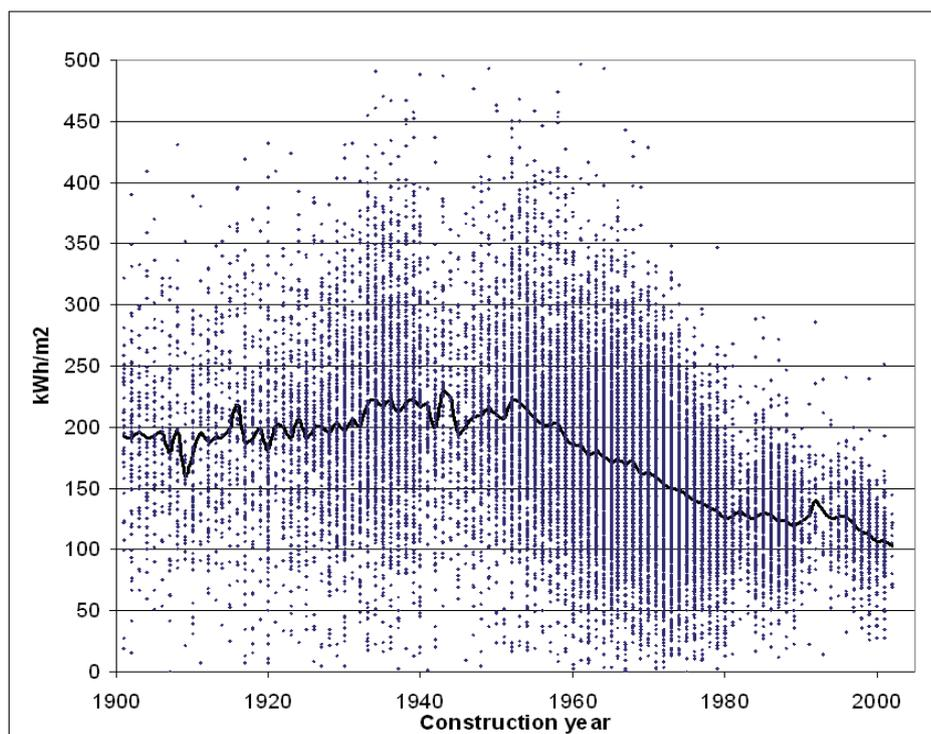
Figure 1. Yearly natural gas consumption kWh/m<sup>2</sup> in 2003 for Danish single-family houses related to construction year and the median. The solid line is the locus of the medians of all the individual observations for each year and the dots are the individual observations.
