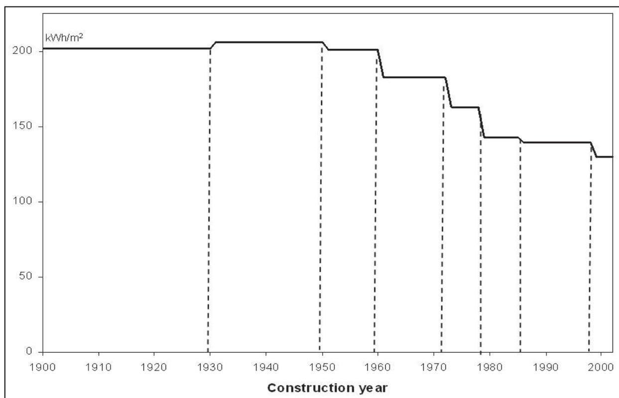
Figure 3. Estimated household natural gas consumption kWh/m<sup>2</sup> per year calculated for a comparable standard house constructed in different periods
