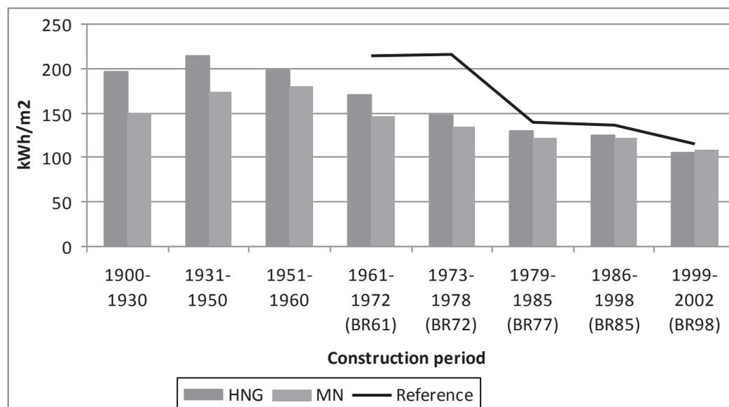
Figure 2. Mean natural gas consumption, kWh/m<sup>2</sup> in 2003 for the houses in our dataset and calculated reference according to U-values in BR.
