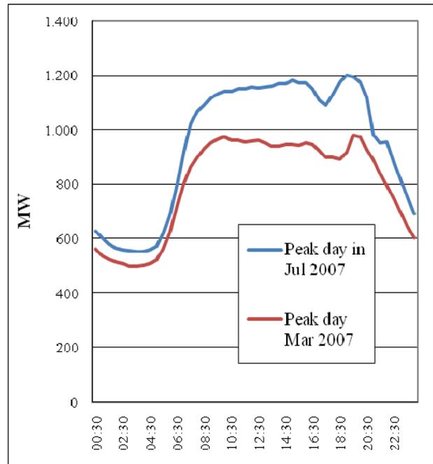
Figure 5: Load curve for Cape Town Metro. Scaled up to cover the complete supply area.
